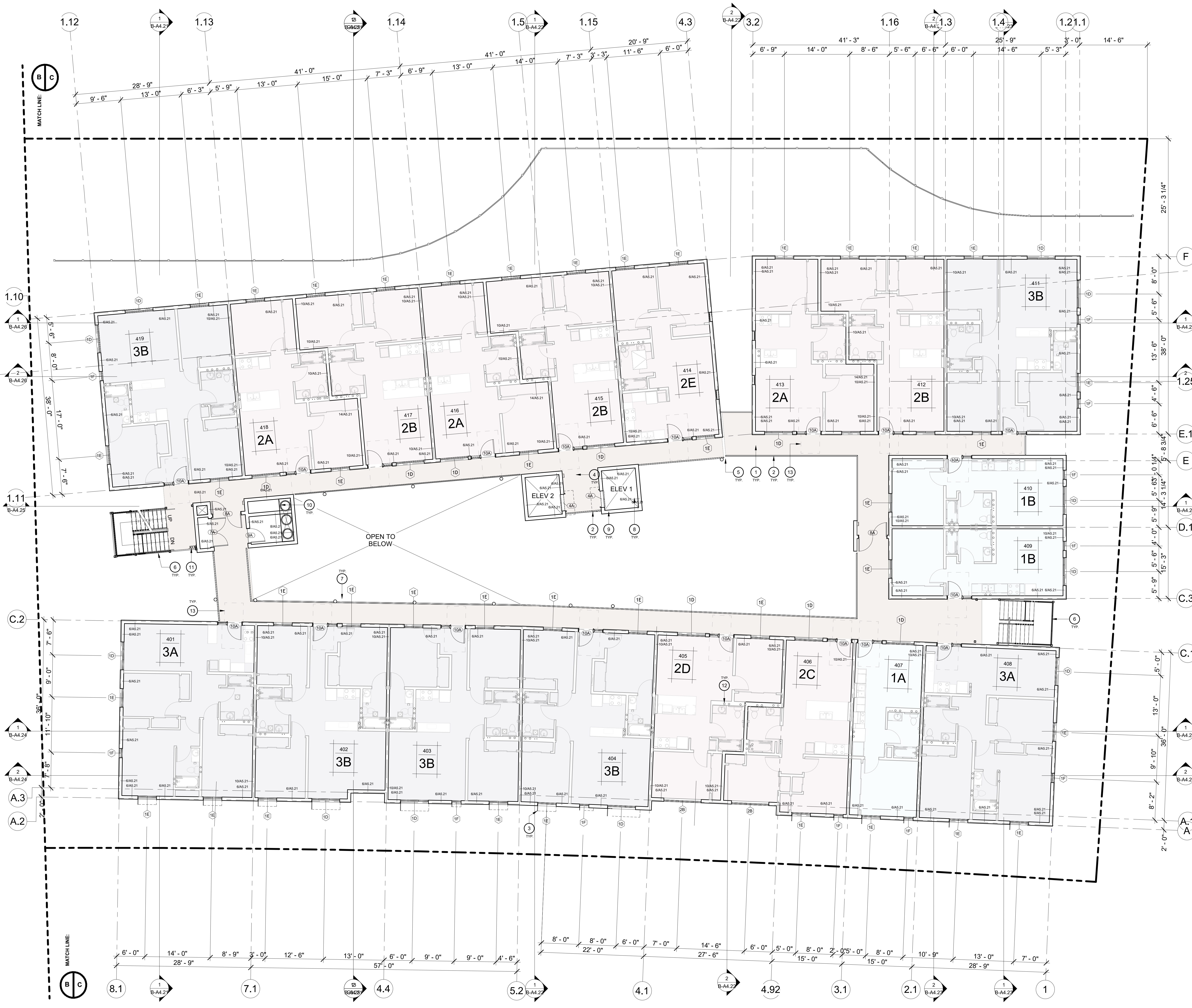
1 BUILDING B - 3RD & 4TH FLOOR PLAN 1/8" = 1'-0"
