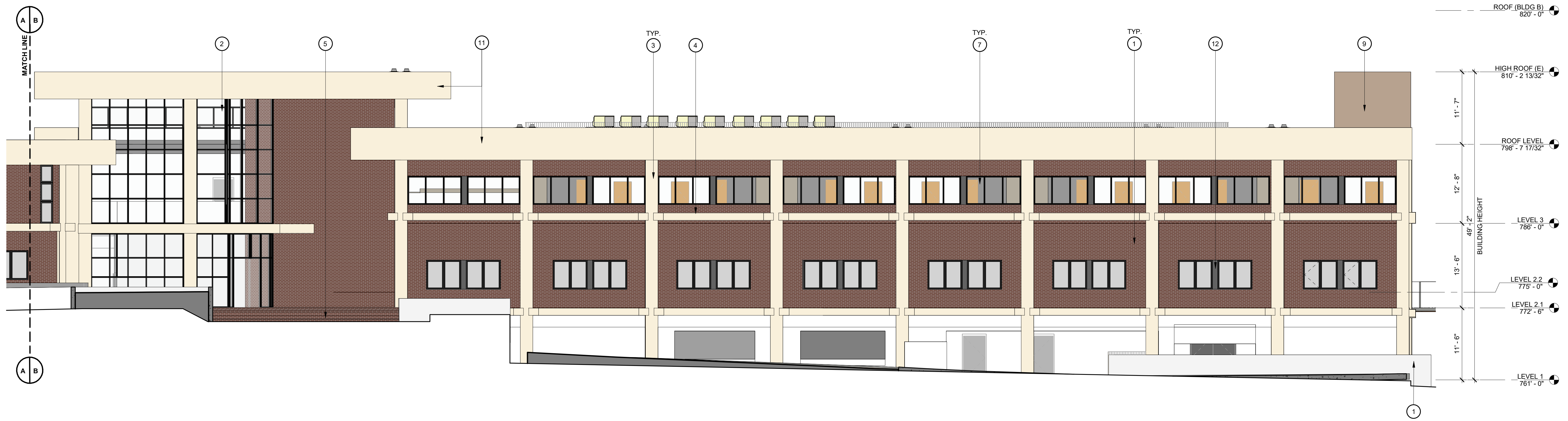
3 BUILDING A (PART 2) WEST ELEVATION 1/8" = 1'-0"
