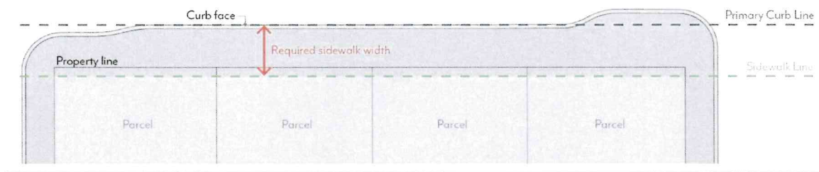
Figure NLSP-3: Sidewalk Line
