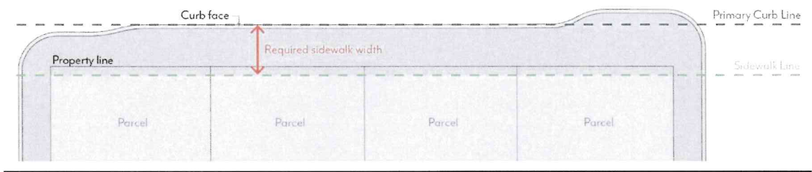
Figure NLSP-3: Sidewalk Line
