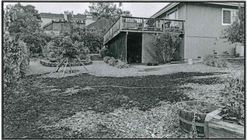
Figure 9: Bark mulch burned up to gravel landscaping adjacent to house during Glass Fire. Note: Homeowner had bark mulch removed and replaced with rock landscaping only two weeks prior to start of Glass Fire.
