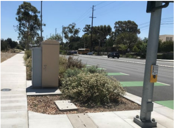
Photo 13 Undergrounding utilities improve sidewalk clearances and help reduce hazards during weather related power outages.
