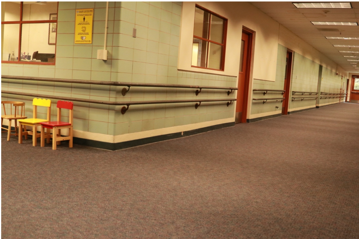
Figure 48. Double-height hand railings optimize accessibility throughout the interior and exterior
