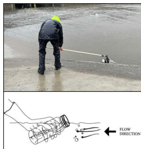
Manual sample collection methods using an intermediate container
