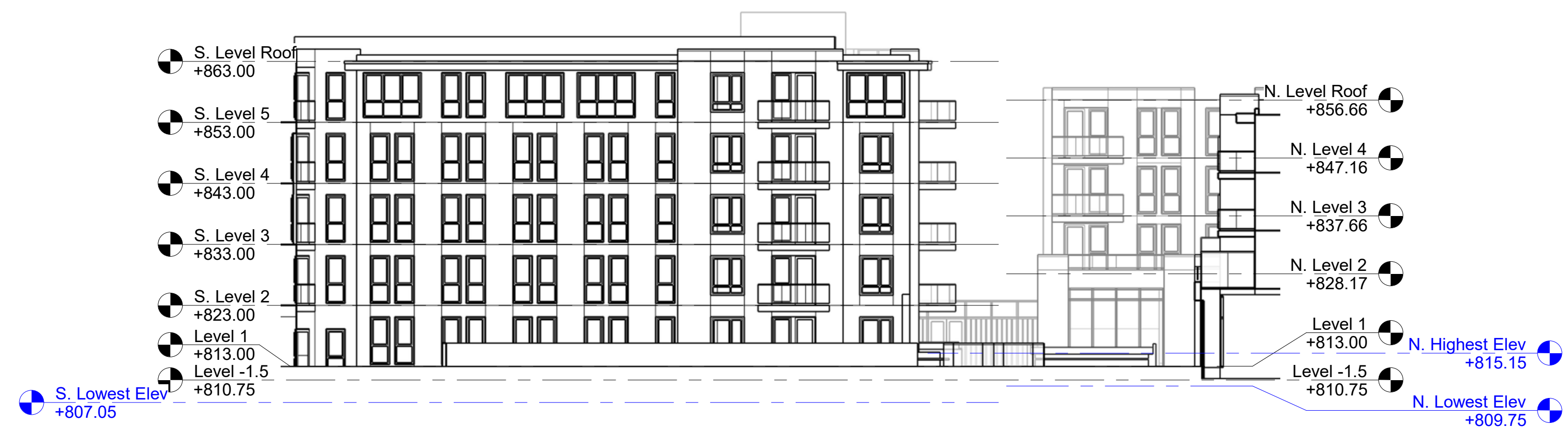
3 Courtyard Elevation (West) B&W 1/16" = 1'-0"
