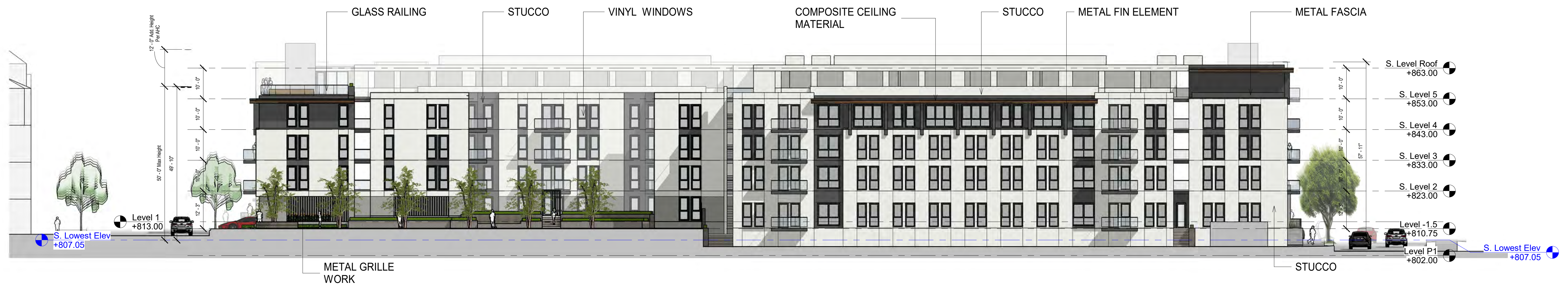
② South Elevation 1/16" = 1'-0"
