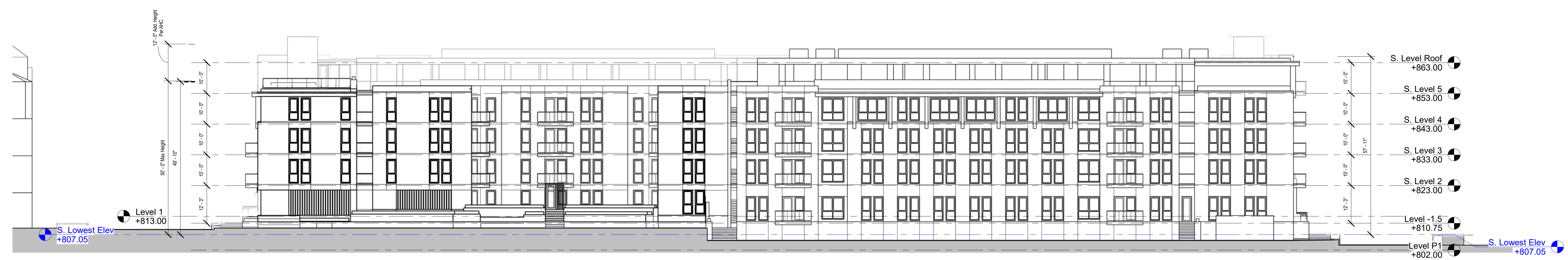
① South Elevation B&W 1/16" = 1'-0"
