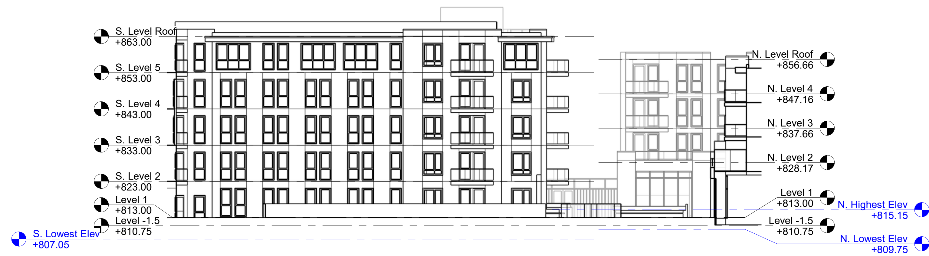
3 Courtyard Elevation (West) B&W 1/16" = 1'-0"
