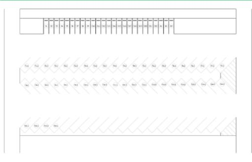
Figure 1. Option 1 Conceptual Site Plan. "5" denotes shuttle bus charging stalls and "T" transit bus.
