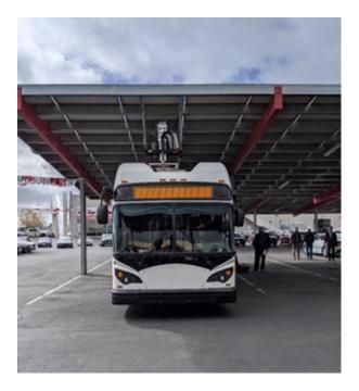
Figure 1-5: In-Depot Overhead Charging Example (Source: CALSTART)
