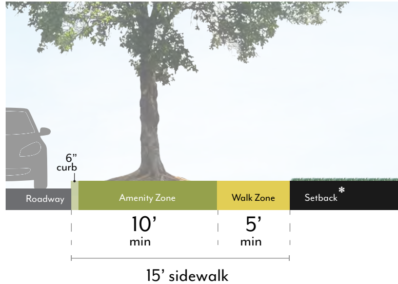
Diagram 7: 15' Sidewalk (Allen Ave. residential)
