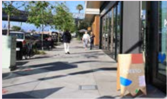
Wider Walk Zones of 7 feet or more are appropriate for commercial retail areas
