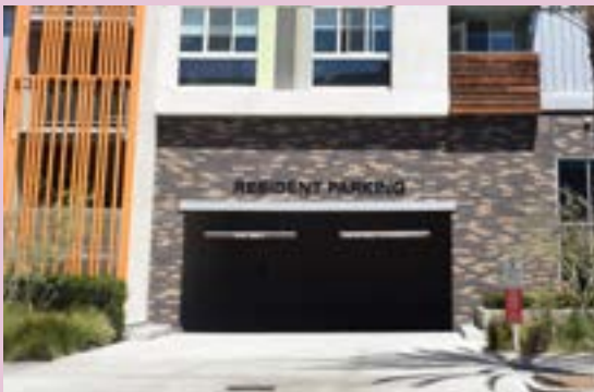
Entrances to structured parking should be integrated into façade design and shall screen upper portions of the entrance not required for vehicle clearance.
