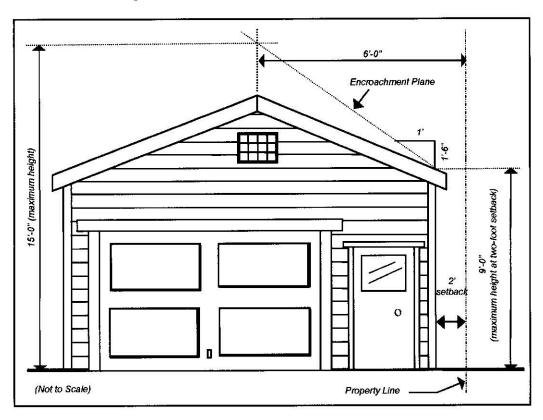
Figure 5-1 - Encroachment Plane and Setbacks for Accessory Structures
