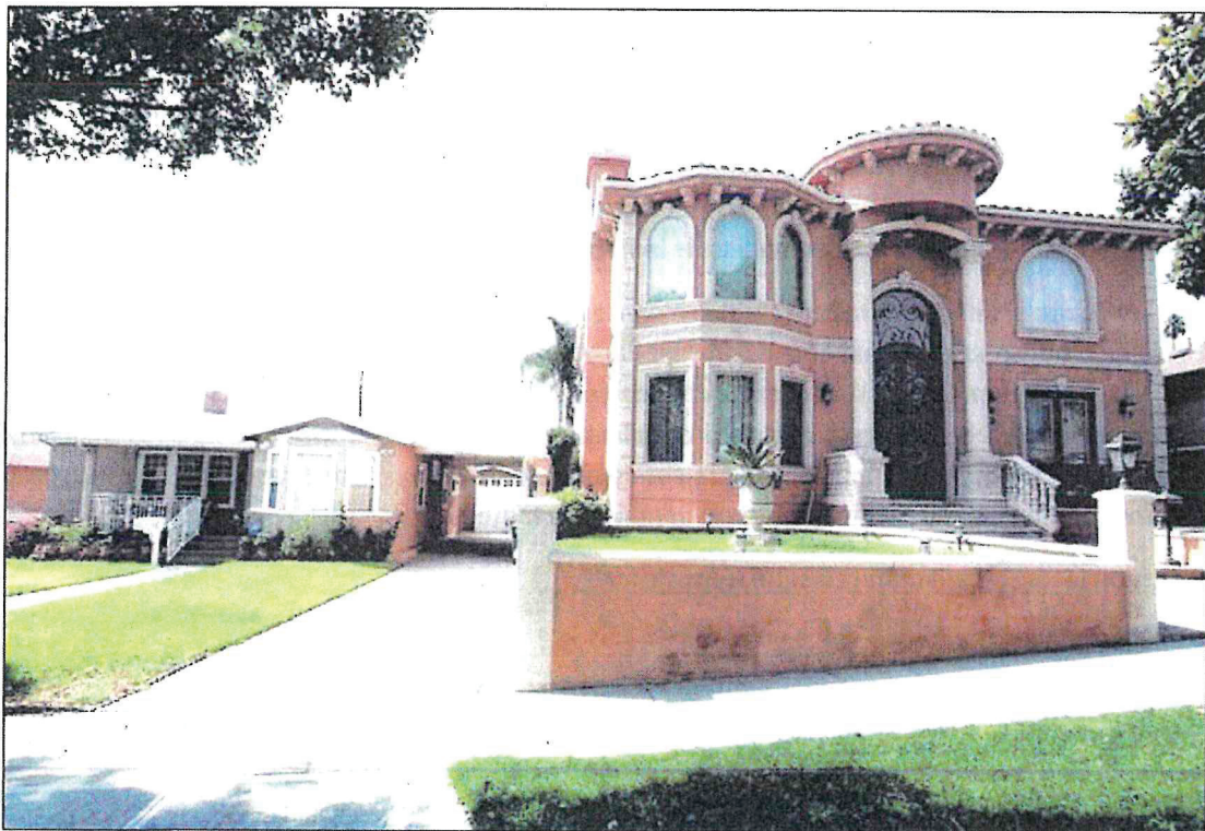
The house at right has a two-story, monumentally-scaled entry that is out of scale compared to the modestly-sized porch and entry of the neighboring house. The house's windows and doors are also disproportionately large.
