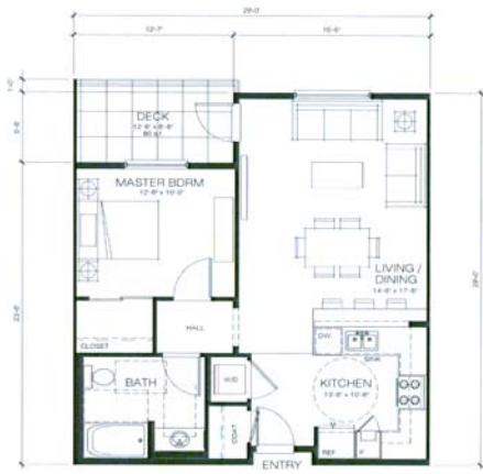
UNIT 3 1 BEDROOM + 1 BATH GROSS UNIT SF = 740 S.F. LIVABLE UNIT SF = 590 S.F. DECK AREA = 90 S.F.
