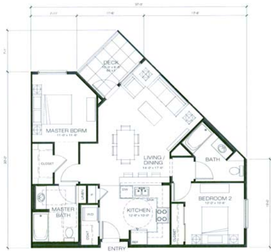
UNIT 5 2 BEDROOMS - 2 BATHS GROSS UNIT SF - 875 S.F. LIVABLE UNIT SF - 719 S.F. DECK AREA - 85 S.F.
