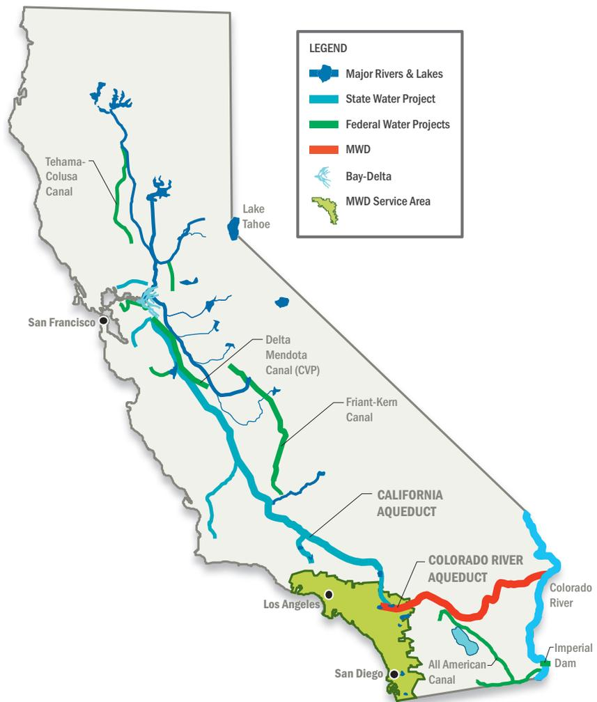
**Figure 2-5. Major Water Conveyance Facilities in California**
