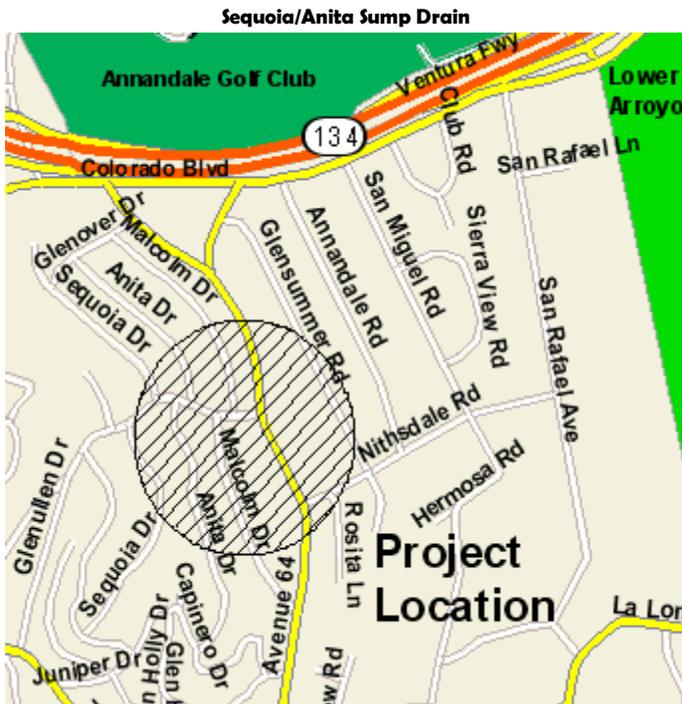
**DESCRIPTION:** This project provides for the construction of a storm drain from Avenue 64 and Nithsdale Road to an existing system in Malcolm Drive north of Glenullen Drive and the reconstruction of portions of the existing system in Sequoia Drive and Anita Drive.
