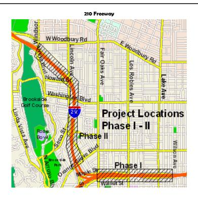
**DESCRIPTION:** This project will provide for the construction of sound walls along a portion of the Route 210 Freeway. Construction of the project will be done in two phases. Phase I includes the east portion of the 210 Freeway between Fair Oaks and Wilson Avenue and will cost approximately \$23,000,000. Phase II includes construction of sound walls on the northern section of the 210 Freeway between Orange Grove and Arroyo Boulevard/Windsor Avenue and will cost approximately \$17,000,000.
