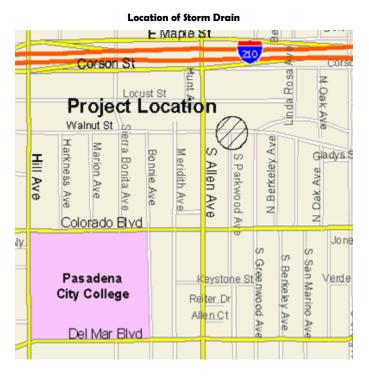
**DESCRIPTION:** This project provides for the replacement of the existing cross-gutter in Walnut Street with a culvert or a storm drain. Construction of a culvert will take the water south to Parkwood Avenue. If a storm drain is selected it will take the runoff 400 feet west to Allen Avenue.
