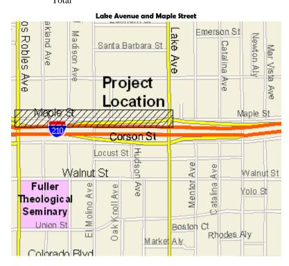
**DESCRIPTION:** This project provides for the restriping of Maple Street to create three throughlanes from Lake Avenue to Los Robles Avenue. Maple Street will be widened within the existing right-of-way to provide the additional traffic lane and to retain the bike lane. Adding this additional lane will involve the following:
