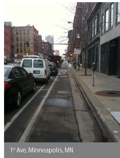
FIGURE 3-5 CURB-SIDE BUFFERED BIKE LANE
