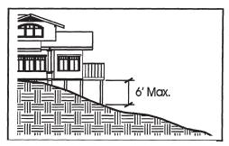
Figure 2-5 – Height Limit for Lowest Floor and Decks
