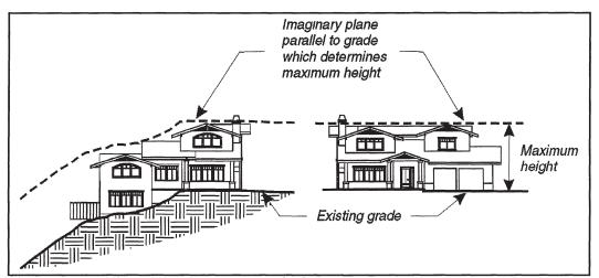
Figure 2-4 – Height Measurement on Hillsides
