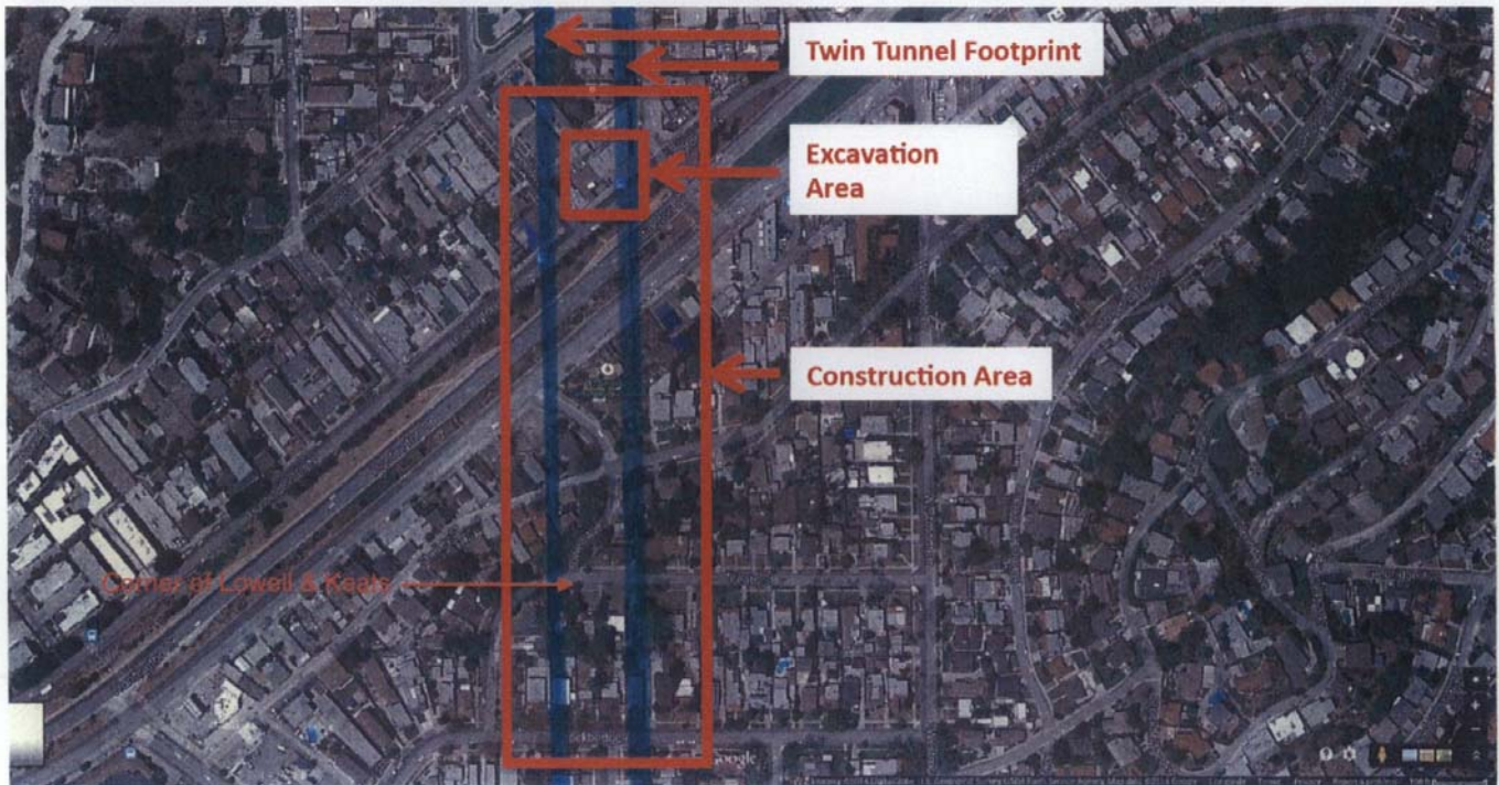
Arial View of East El Sereno showing an example of a TBM breakdown and Associated Construction Area
