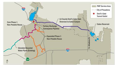
Tertiary treated indirect potable reuse: This concept involves conveyance of tertiary-treated recycled water to Eaton Canyon
