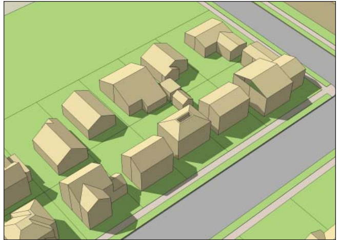
A historic/sensitive context. Buildings are consistently set back from the street, have similar building lengths along the street frontage, and share similar heights and massing.
