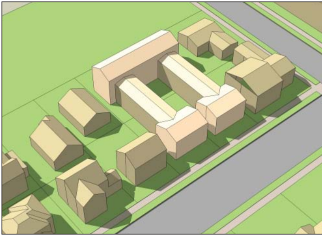
A new building is introduced into a historic/sensitive context. Despite its large size, the new building's massing and setback along the street is similar to those of its neighbors.
