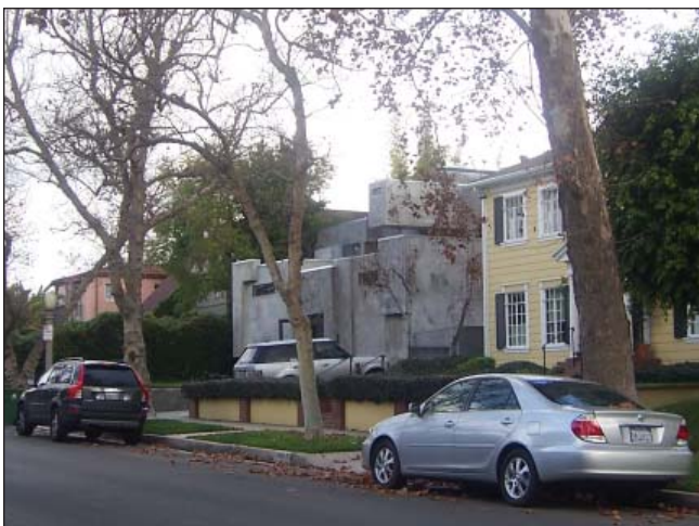
⚠ A multi-family building that, through its massing, window placement, and street-facing predominantly blank wall, is insensitive to its historic/sensitive context.
