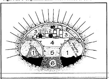
Figure ES-3 Sequential Excavation Method of Construction
